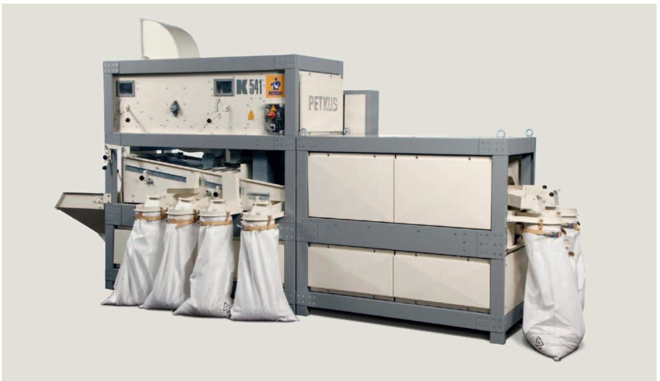
The **PETKUS seed cleaner K 541** is used for high-quality seed cleaning of free flowing bulky products, e.g. grain, oilseeds, fine seeds (grass and vegetable seeds). The high standard of cleaning is achieved by a combination of the screening process, the air aspiration system, and the indented cylinders.
