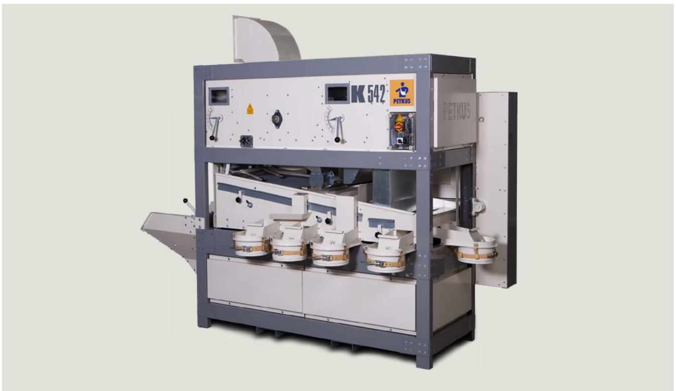
The **PETKUS Seed Cleaner K 542** is used for high-quality seed cleaning of free flowing bulky products, e.g. pulses which do not need to be processed with an indented cylinder. Furthermore, the seed cleaner can also be used for the intensive cleaning of grain, oilseeds, and pulses. The high standard of cleaning is achieved by a combination of the screening system and the air aspiration.
